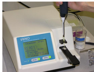
Vapor pressure osmometer ensures all extenders are osmotically balanced.
